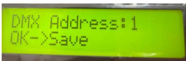
The first channel is brightness, brightness channel values 0-3 corresponding to 0 (not bright), 4-7 corresponding to 1, 8-11 corresponding to 2 252-255 corresponds to 63.
